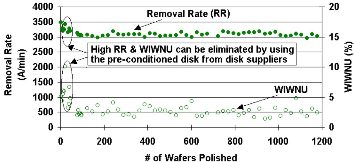
Fig. 2. Thermal oxide polishing removal rate and within wafer non-uniformity as a function of number of wafers polished using a new conditioning disk. (1) Pressure (psi): 5/5.8/5 membrane/retaining-ring/inner tube. Others: the same as Fig.1.
