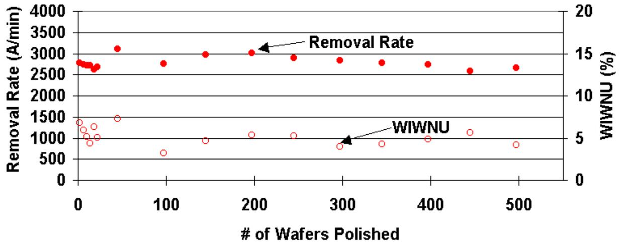
Fig. 3. Thermal oxide polishing removal rate and within wafer non-uniformity as a function of number of wafers polished using a conventional conditioning disk. (1) Pressure/others: the same as Fig. 1.
