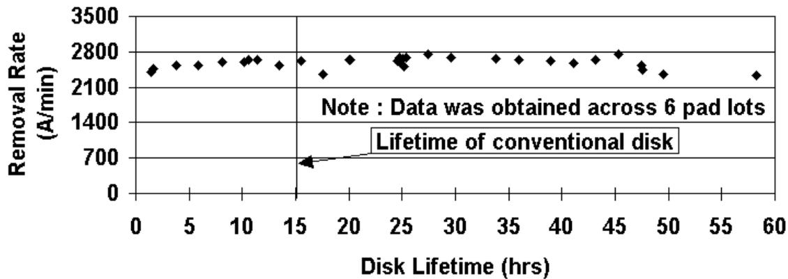
Fig. 1. Thermal oxide polishing removal rate as a function of disk life for a new conditioning disk. Pressure (psi): 4/4.6/4 membrane/retaining-ring/inner tube. (1) Speed (rpm): 93/87 platen/head. Slurry: SS12. Slurry flow rate: 200 ml/min. Pads: IC-1000/Suba IV, K-groove and 50 mm thick.
