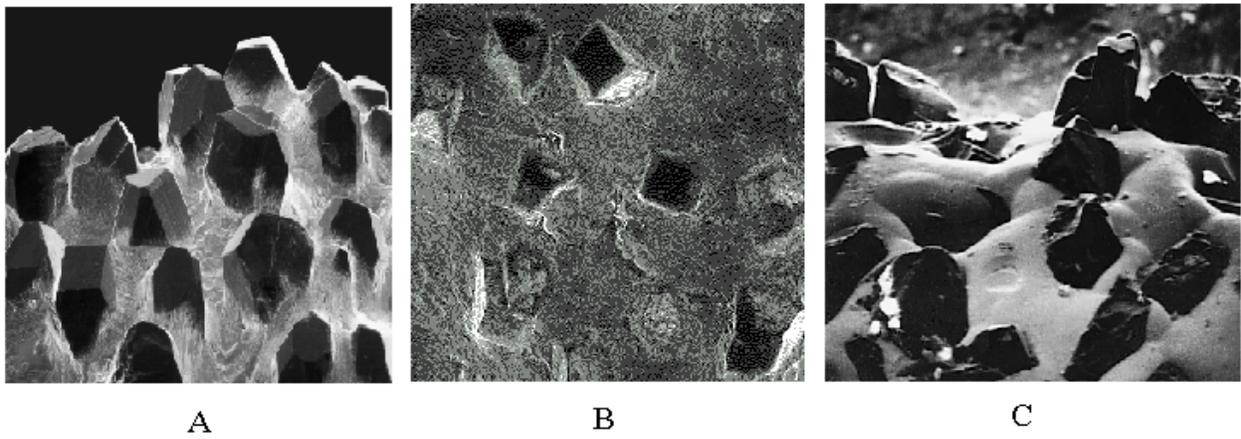
Fig. 4. SEM micrographs of a new diamond disk (tilted view) before pad conditioning [A], a new diamond disk (top view) after pad conditioning [B], and a conventional diamond disk (tilted view) before pad conditioning [C]. (1)
