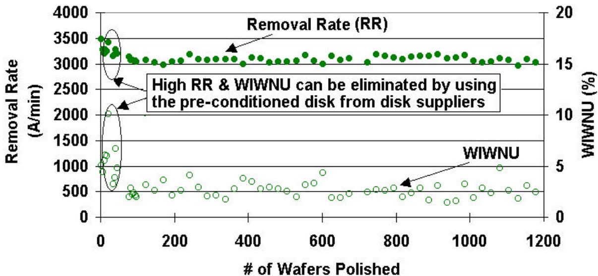
Fig. 2. Thermal oxide polishing removal rate and within wafer non-uniformity as a function of number of wafers polished using a new conditioning disk. Pressure (psi): 5/5.8/5 membrane/retaining-ring/inner tube. Others: the same as Fig.1.
