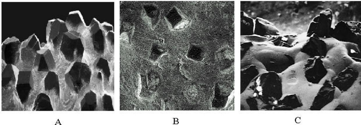
Fig. 4. SEM micrographs of a new diamond disk (tilted view) before pad conditioning [A], a new diamond disk (top view) after pad conditioning [B], and a conventional diamond disk (tilted view) before pad conditioning [C].
