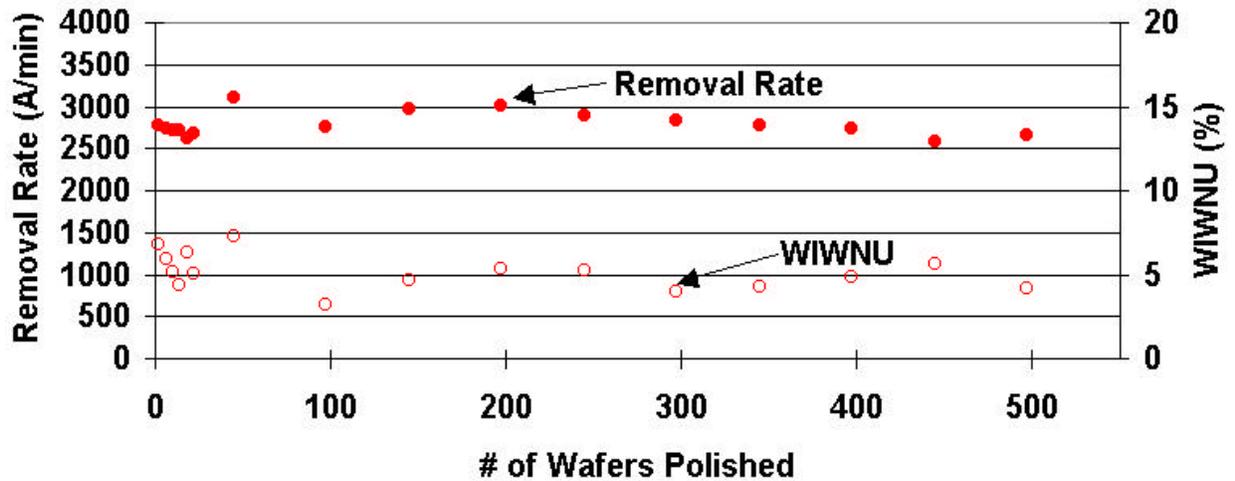
Fig. 3. Thermal oxide polishing removal rate and within wafer non-uniformity as a function of number of wafers polished using a conventional conditioning disk. Pressure/others: the same as Fig. 1.
