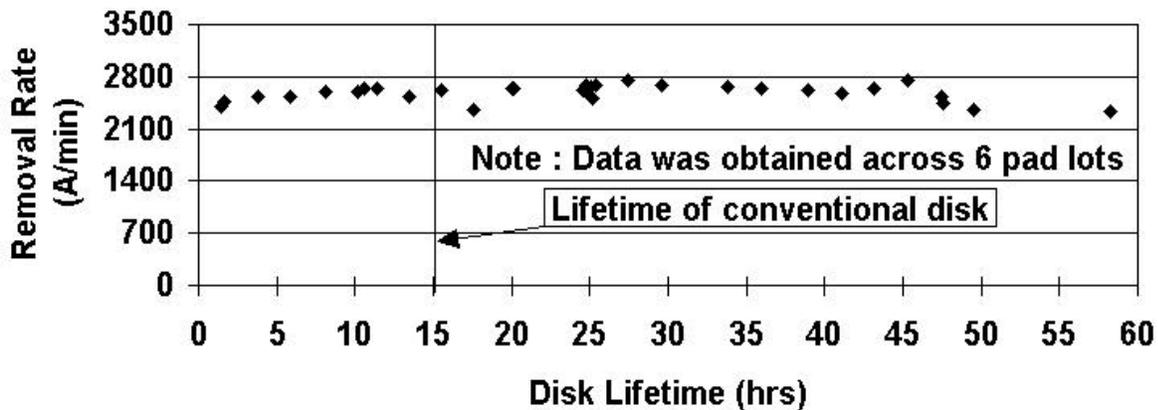
Fig. 1. Thermal oxide polishing removal rate as a function of disk life for a new conditioning disk. Pressure (psi): 4/4.6/4 membrane/retaining-ring/inner tube. Speed (rpm): 93/87 platen/head. Slurry: SS12. Slurry flow rate: 200 ml/min. Pads: IC-1000/Suba IV, K-groove and 50 mm thick.
